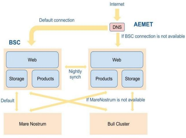
Figure 2: Configuration of the BDFC systems
